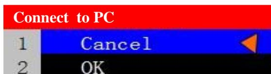
If you select “OK” option within 5 seconds, the camera will be recognized by your PC as a removable disk and will suggest a software application on your PC to be used to view your video files.
